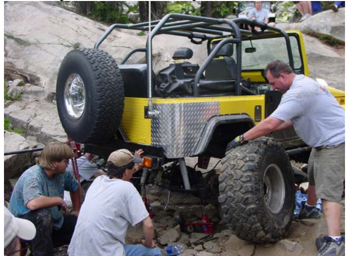
Twisted pinion shaft under repair...
